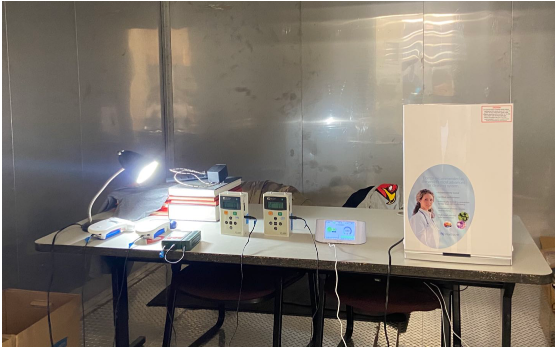
Figure 1. Inside chamber set up for the air cleaner CADR tests
