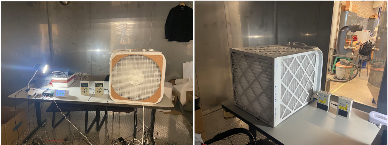
Figure 1. Inside chamber set up for the air cleaner CADR tests
